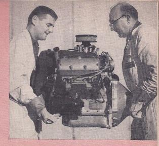
connecting rods, crankshaft, valve train, timing gears, flywheel and fan pulley are made of iron or steel. Cylinders are made of die-cast porous aluminum so the metal will absorb and retain oil to cut friction. They are chrome-plated to reduce wear. Piston rings, of iron, are unplated.
